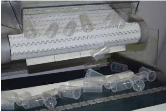
Fig 3.1. Fully automatic Specimen Container production line - Container feeding.
