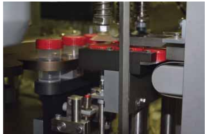
Fig 3.4. Fully automatic Specimen Container production line - Container / cap closure.
