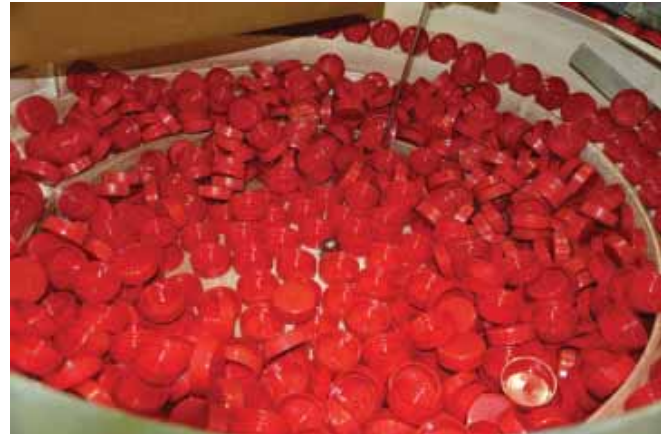
Fig 3.2. Fully automatic Specimen Container production line - Cap feeding.
